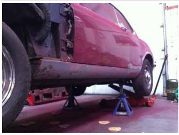
*Sill and rear wing repairs underway.*
