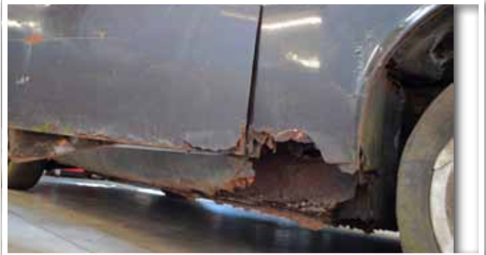
Corrosion has taken its toll on the bodywork and internal structures after so long being neglected
