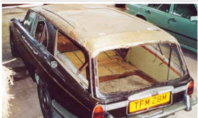
The roof is a remarkable pressing with a scalloped area surround a bit like a contemporary Triumph 2000 estate car.
