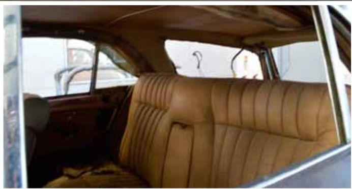
The rear seat back has kept in remarkably good condition, although the frame is altered from original. Note the roof with plenty of headroom and rear loading height.
