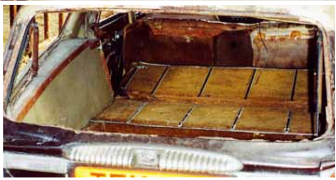
With the rear seat folded down, the loading area is massively extended. The horizontal line across the rear of the roof is where the tailgate opens from providing plenty of access, a well thought out feature.
