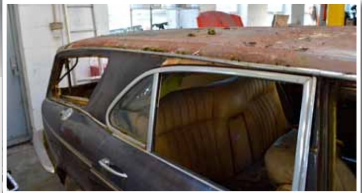
With the roof covering stripped away, Keith has been unable to find a join, suggesting that the roof pressing was a complete one-off pressing especially for the car.
