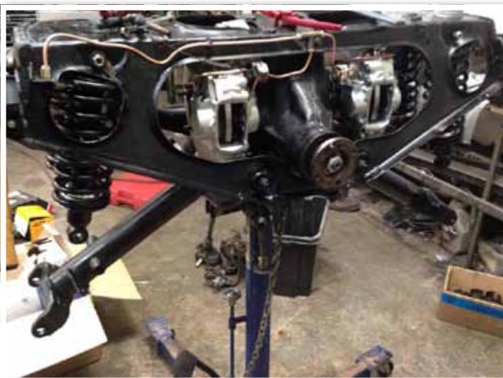
The rear suspension overhauled and refurbished ready for re-assembly onto the car.
